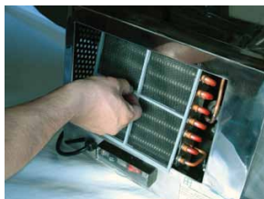
Step 3-2. Take out the AIR FILTER from the condenser
