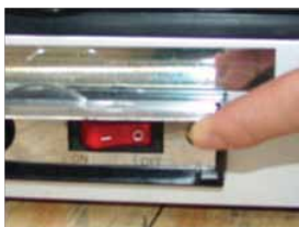
1. Hold the fuse holder and turn CCW to unscrew
