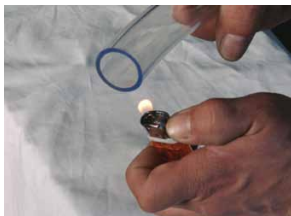
STEP 3-2: Make soft the end of the Tube with the Lighter. (CAUTION: Do NOT overheat)
