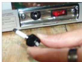
2. Remove the blown-out fuse from the fuse holder
