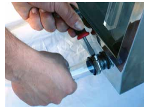
STEP 3-4: Check up if the Tube is completely set onto the Drain Hole.
